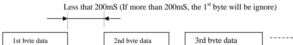
The CAT control program you are writing must construct the 5-byte block, by selecting the appropriate instruction opcode, organizing the parameters, if any, and providing un-used (dummy) argument bytes for padding the block to its required 5-byte length (the dummy bytes can contain any value). The resulting five bytes are then sent, opcode last, from the computer to the **VR-5000** CPU via the serial port and CAT jack on the radio rear panel.
