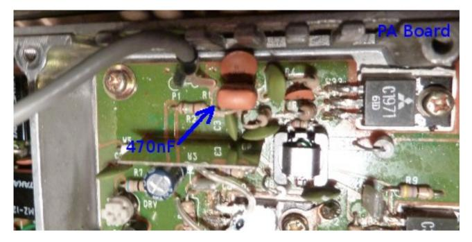
PA board coupling capacitor modification
